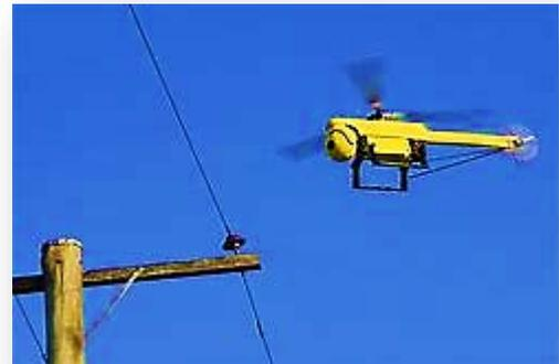
Increasingly, UAVs or Drones are being used to inspect powerlines. Avista plans to deploy this technology as part of Wildfire Resiliency.
