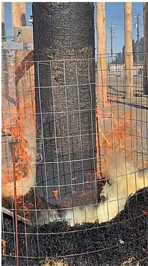
*On March 3<sup>rd</sup>, 2020, Avista conducted a field test of the Genics Fire-Mesh product. An FR wrapped pole was subjected to a 30-minute fire and sustained only minor damage. Unlike FR paint, this mesh product does not require on-going maintenance and can be applied much more easily than paint.*
