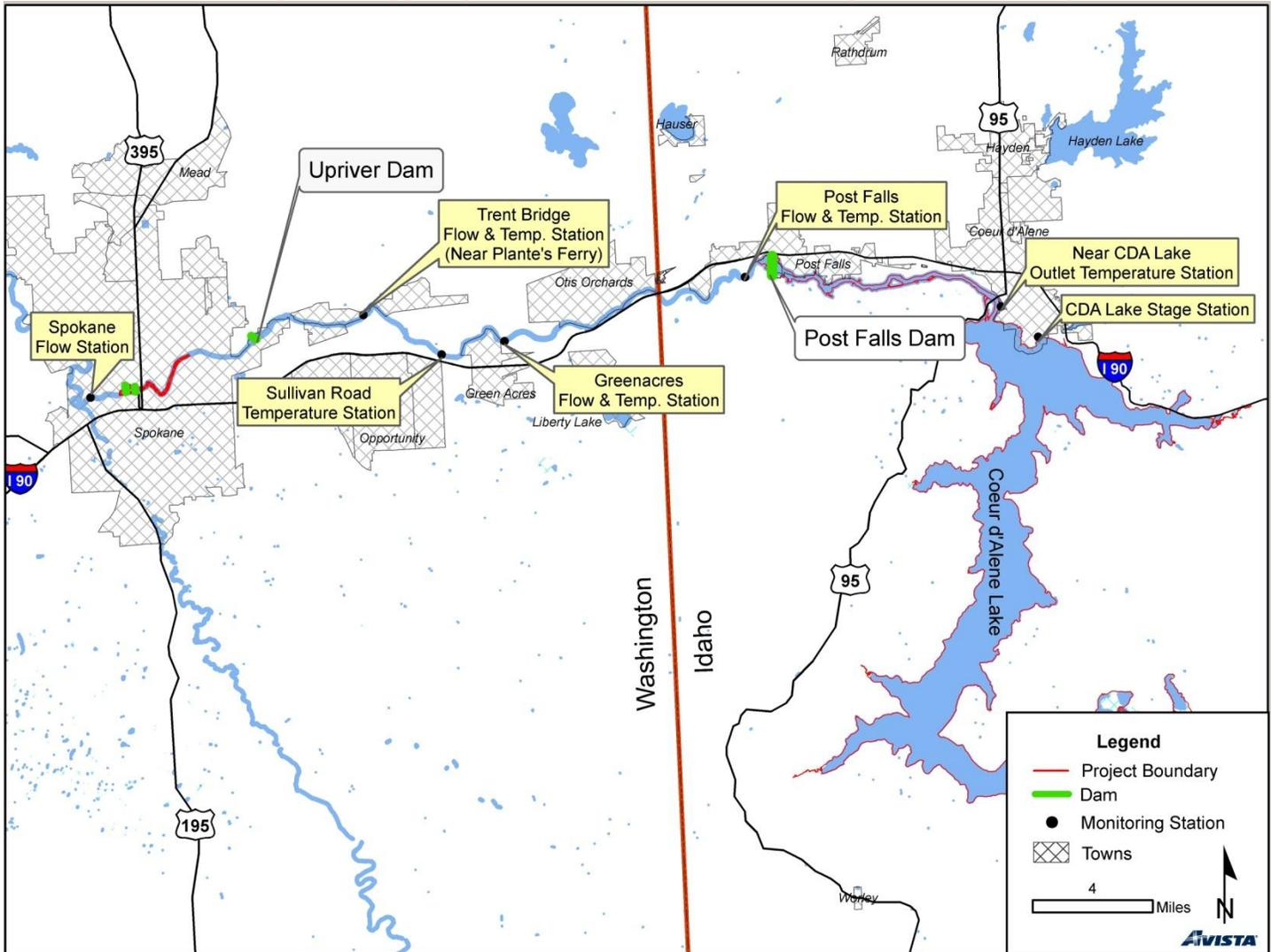
During about half of any year, a natural channel restriction controls Coeur d'Alene Lake's water elevation and Spokane River flows. In contrast, the Post Falls HED controls water elevations in Coeur d'Alene Lake and flow in the Spokane River after spring run-off, and through the summer and fall.
