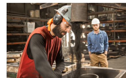
Custom molds are formed using sand and self-hardening chemicals (shown here).
