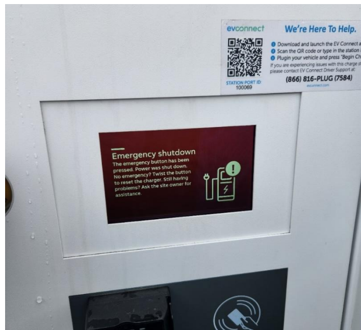
Figure 17: Emergency stop message displays on station after driver left the e-stop engaged after a session.
