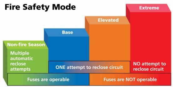
A permanent fault (circuit that won't close automatically) requires thorough inspection before reclosing the circuit. This additional step may extend the duration of a outage.
