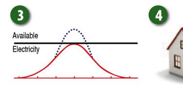
Home uses electric heat at lower off-peak rate under normal conditions. Electricity demand exceeds current power supply and economical energy purchases are not available. Load control is used to avoid uneconomical energy purchases and maintain system reliability. Home is automatically switched from electric to backup heating source. No change in comfort should be noticed between the two systems.
