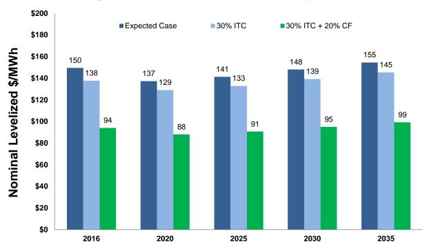
Figure 9.2: Solar Nominal Levelized Cost (\$/MWh)
