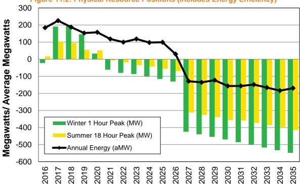
Figure 11.2: Physical Resource Positions (Includes Energy Efficiency)
