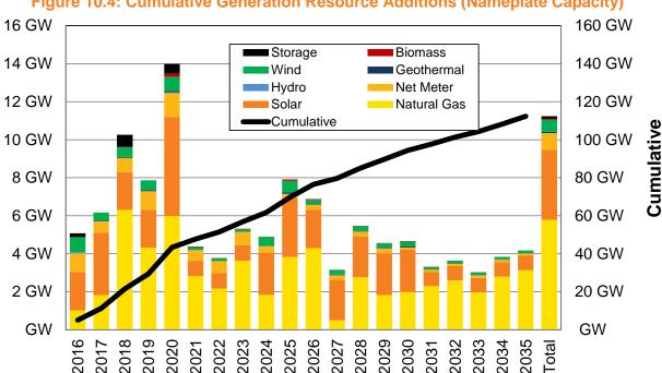
Figure 10.4: Cumulative Generation Resource Additions (Nameplate Capacity)
