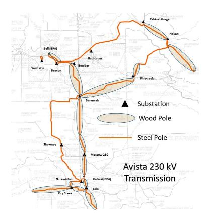
Avista's 230 kV system was initially built in the late 1950's and early 1960's, after the construction of the Noxon Rapids and Cabinet Gorge dams. In 2003, portions of the system were upgraded as part of the West of Hatwai agreement with Bonneville Power. Several wood lines were converted to steel during that time period including:
