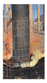
On March 3<sup>rd</sup>, 2020, Avista conducted a field test of the Genics Fire-Mesh product. An FR wrapped pole was subjected to a 30-minute fire and sustained only minor damage. Unlike FR paint, this mesh product does not require on-going maintenance and can be applied much more easily than paint.
