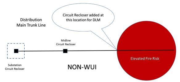
By adding circuit reclosers at strategic locations, Avista Distribution Operations can re-task those devices during periods of elevated fire danger to operate in fire protection mode rather than reliability mode. A proposed scheme is illustrated in the block diagram below.
