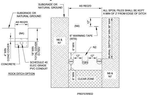
Figure 4.1 - Service Ditch Detail
