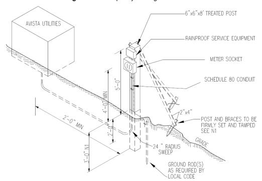
Figure 2.3 – Temporary Underground Service
