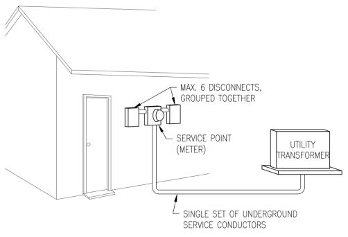
Figure 1.3 – A Single Overhead Service with Multiple Meters
