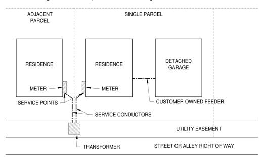
Figure 1.7 – Acceptable Service Configuration for a Multi-Family Residence on a Single Lot \*
