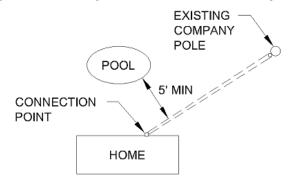
Figure 4.9 – Underground Clearances for New Developments
