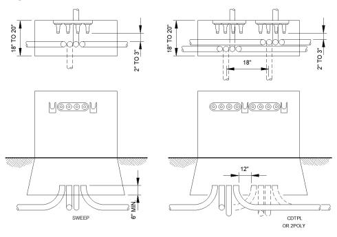
Figure 4.26 – Conduit Entrance for 3- Phase Padmounted Junction Enclosures
