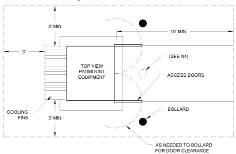
Figure 4.27 – Bollard Clearances
