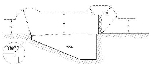
Figure 3.10 – Clearances Around Swimming Pools and Hot Tubs
