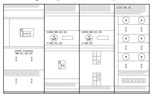
Figure 5.5 – Typical Switchboard Multi-Meter Layout
