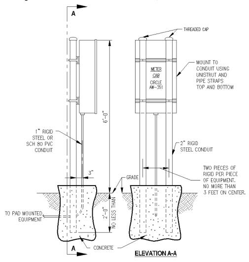
Figure 4.21 - Pedestal Mounted Meter Enclosure, Dedicated Transformer
