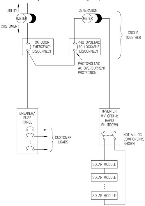
Figure 6.4 – Generation Production Meter and Disconnect Location
