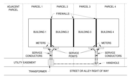
Figure 1.9 – Acceptable Service Configuration for an Apartment Complex that may be Converted to Townhomes in the Future \*
