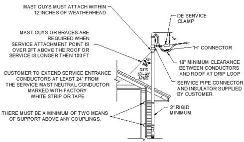
Figure 3.2 - Overhead Roof Mast Above Eave
