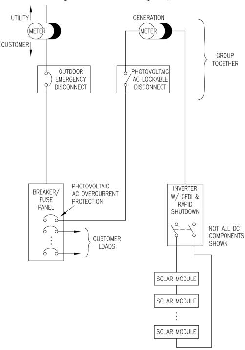
Figure 6.2 – Solar One-Line Diagram Option B
