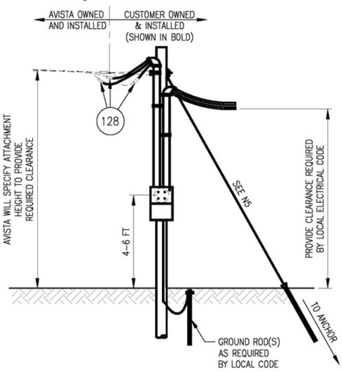
Figure 3.6 - Overhead to Underground Service Pole
