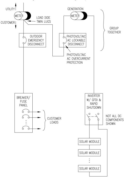
Figure 6.3 - Solar One-Line Diagram Option C
