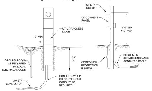
Figure 4.12 - Underground Service Pedestal
